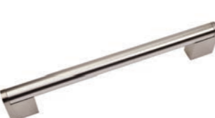
H264 Round Bar Handle Stainless Steel 200mm Long x 14mm Thick 160mm Centres | 34mm Projection
